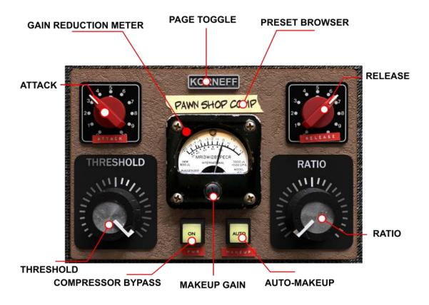
**ON** - press this to engage the compressor circuit. If you switch this off, the compressor is bypassed. Your signal will still go through the tube signal path, so you can use the Pawn Shop Comp as a just a preamp and EQ.
